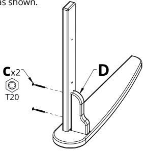
**5.** Repeat step 1-4 with Parts B, C & D. These assemblies will be used in step 7.
