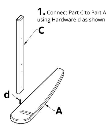
**2.** Rotate Part C clockwise until tight in the orientation shown
