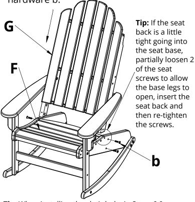
**Tip:** When installing the chair bolts in Steps 6 & 7, insert the bolt into the hole, align it with the nut and finger-tighten the bolt a couple of turns into the nut before driving with a drill. This will help to reduce the risk of cross-threading.
