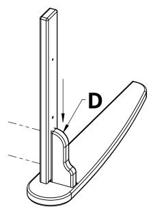
**4.** Using Hardware c attach Part D as shown.
