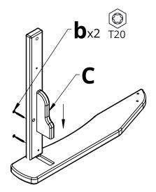
**2.** Place Part C into the precut slot and attach it using Hardware b
