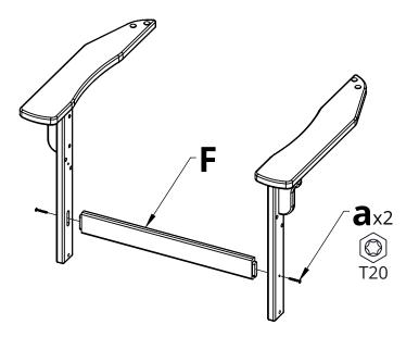
**4.** Attach Part F to the previous assemblies using Hardware a
