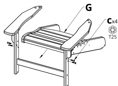
**5.** Place Part G between the previous assemblies & attach it using Hardware c
