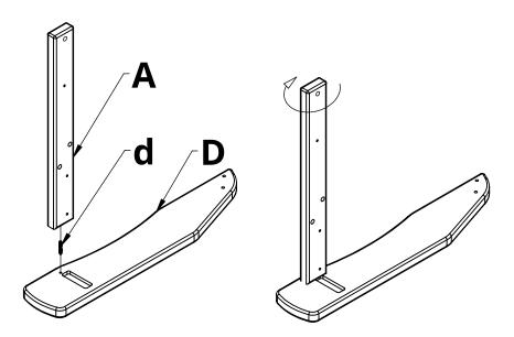
**1.** Attach Part A to Part D by inserting Hardware d into the pre-drilled holes and rotating Part A clockwise, stopping when the assembly is tight
