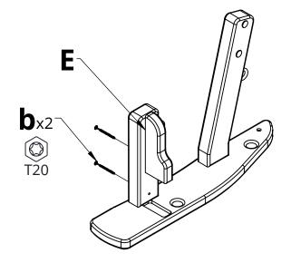
**2.** Place Part E into the pre-cut slot & attach it with Hardware b
