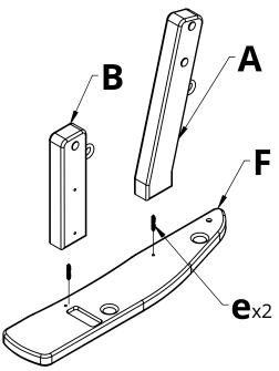
**1.** Attach Parts A & B to Part F by inserting Hardware e into the pre-drilled holes and rotating clockwise, stopping when the assembly is tight
