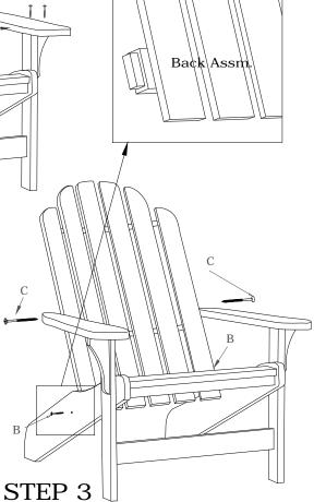
Fit Back Assembly into mortise pockets on insides of Base Assembly. Secure with screws (B) as shown. Attach Arms to seat back using Large Head Screws (C).
