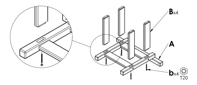
**2.** Place second Part A on assembled piece from Step 1, attach with Hardware b
