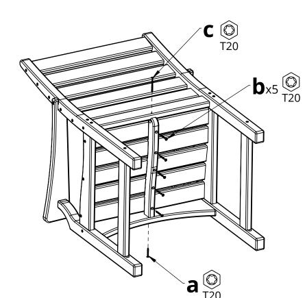
**6.** Connect Part D to the center, underside of Part B as shown
