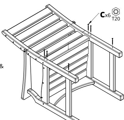
**5.** Turn the assembly over & attach the hardware shown
