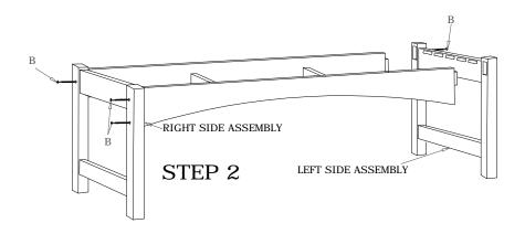
Place Seat Supports in place and using screws (A), attach the Rails as shown in the drawing
