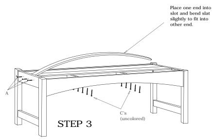
Fit slats into table as shown. From the bottom side use uncolored screws (C) to secure slats. Use screws (A) to attach Side Assemblies to Slats.
