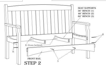
Attach Side Assemblies to Back Assemblies using screws (B) as shown.
