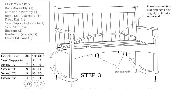
Fit seat slats into bench as shown. From the bottom side use uncolored screws (C) to secure slats. Use screws (A) to attach Side Assemblies to Slats. Attach Rockers with screw (D) from bottom.
