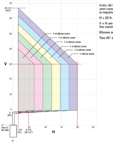
V+H≤ 40 ft. (For longer vent runs, a power vent is required).
