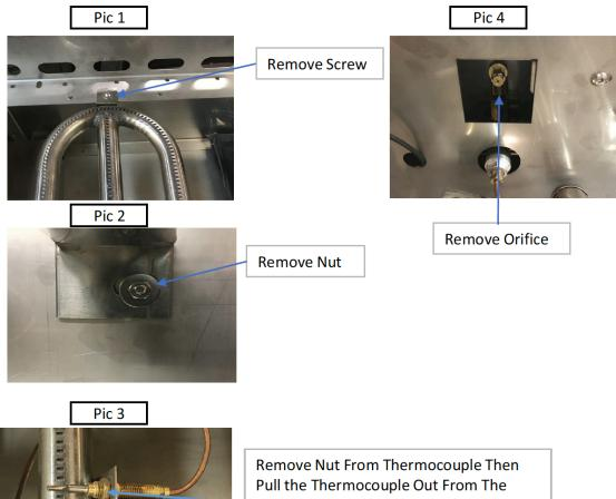
Pull the Thermocouple Out From The Bracket. Note the Position of The Tip of The Thermocouple Before Doing So.
