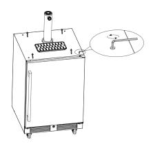
Using the 3mm Allen wrench included with the kegerator, remove (4) M5\*10 screws from the top of the kegerator.
