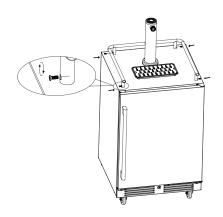
Secure the Drink Guardrail in place with (4)  $\phi$ 9\*22-M5 screws included in the hardware package and tighten them using the Philip Screwdriver.
