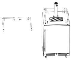
Assemble the two Drink Guardrail sections together and place over the (4) threaded posts.
