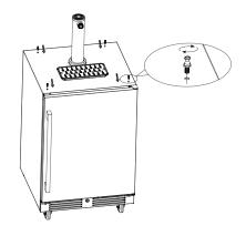
Install (4) threaded posts from the Drink Guardrail hardware package into the screw holes on top of the kegerator.
