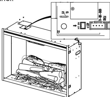
**! NOTE:** If heater button is pressed when heater is permanently disabled, H-- will be displayed.
